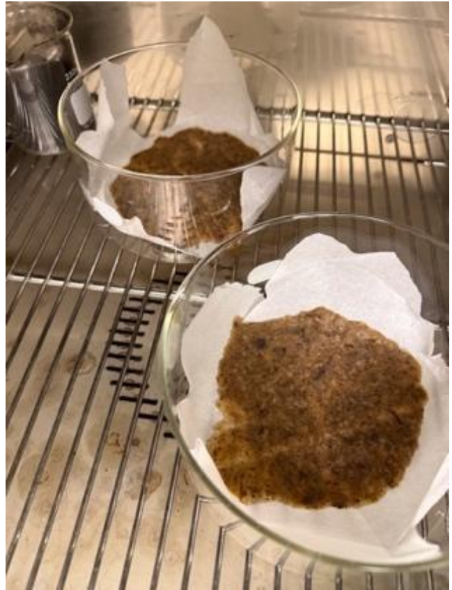
Figure 5. Banana peel paste mixture heated in an oven at 150°C for 45 minutes.
