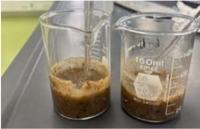
Figure 3. Mixture of banana peel paste, HCl, glycerol, NaOH, and cornstarch stirred in a 400 mL beaker.
